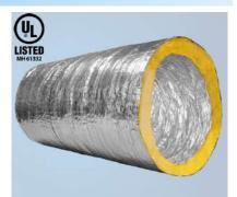
Good quality fiber glass insulation & inner core is double layer of ALU PET & clear polyester permanently bonded with flame retardant bonding adhesive with coated steel spring helix.
