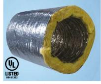
layer is of Good quality fiber glass insulation with BGT facing & inner core is perforated double layer of ALU PET & clear polyester permanently bonded with flame retardant bonding adhesive with coated steel spring helix.
